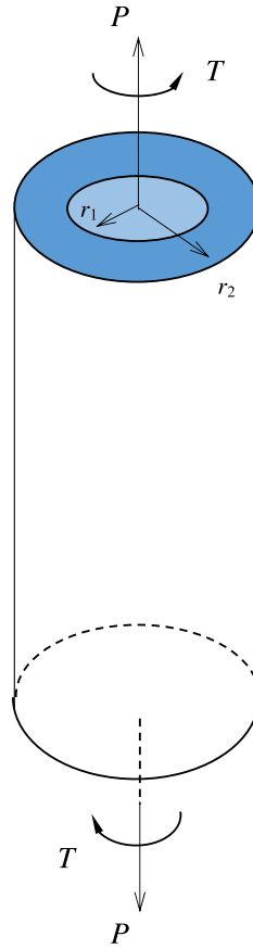
Fig. 1. A bilayered cylindrical composite, with surfaces located at the radial coordinates, r = r_i, i = 1, 2 , under combined torsion T and axial loading P .
