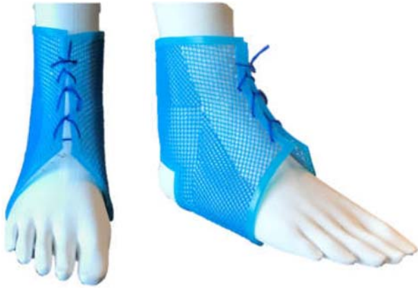
Fig. 10 Fabricated ankle brace with optimized geometric structures
